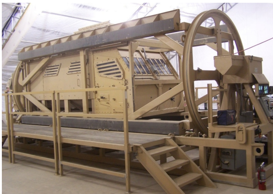
Figure no. 2: A rollover simulator
